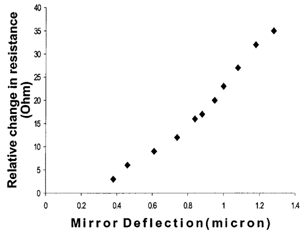
Fig. 16. Plot of CMOS micromirror deflection as a function of relative change in resistance of a single piezoresistor.
